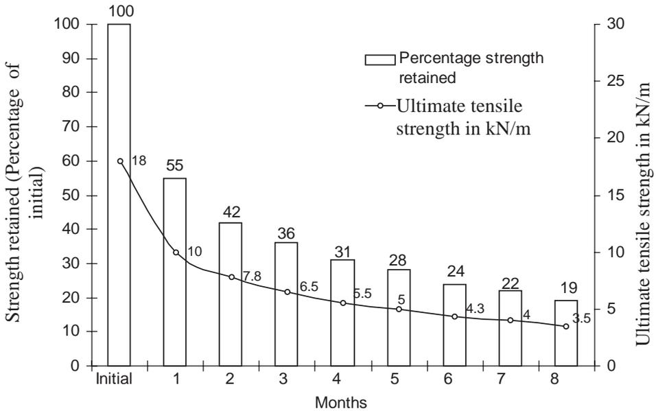
Fig. 6. Variation in the ultimate tensile strength of the coir net after field application.
