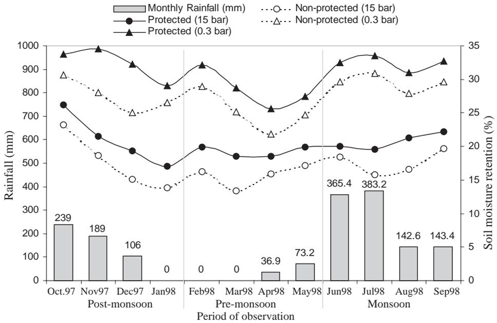
Fig. 3. Comparison of soil moisture retention in protected and non-protected slopes.
