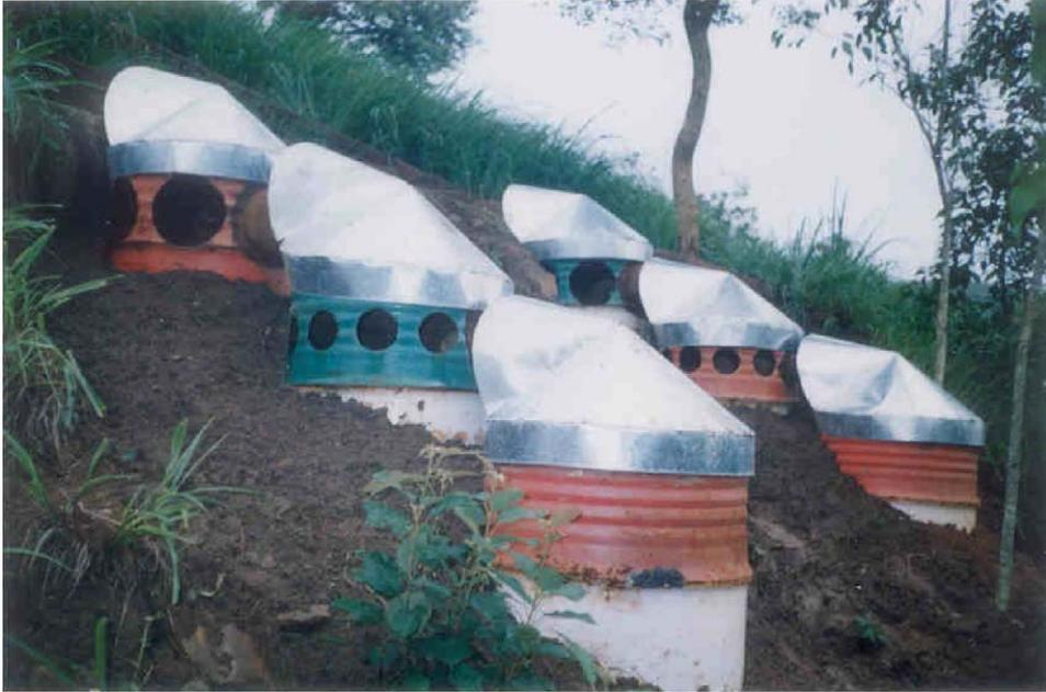
Plate 1. Drum arrangement for collection of runoff and erosion debris from control plots.
