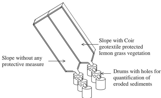
Fig. 1. Schematic of test plots with arrangements for collecting runoff and erosion debris.
