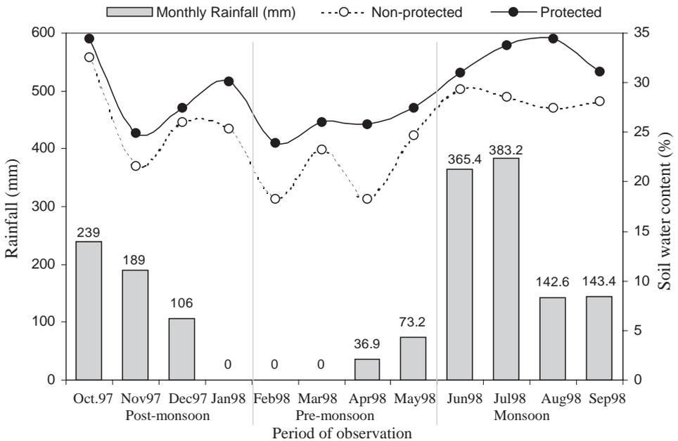
Fig. 4. Comparison of soil water content in protected and non-protected slopes.
