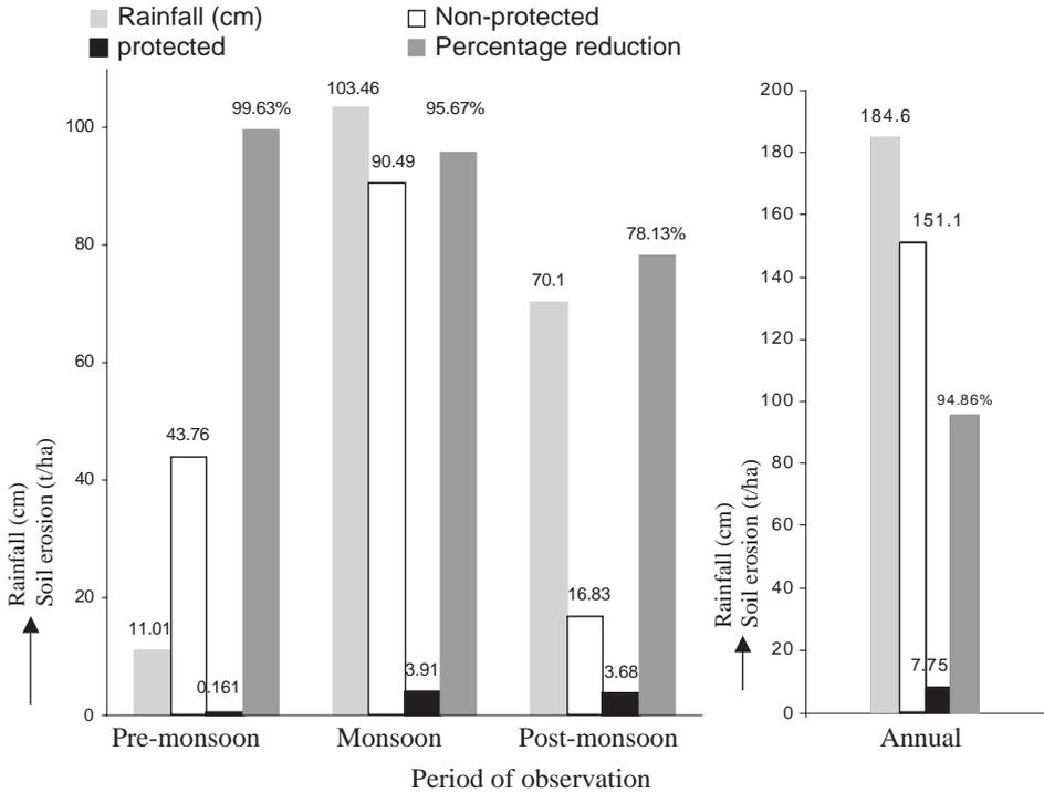
Fig. 2. Comparison of seasonal and annual soil erosion in protected and non-protected slopes.
