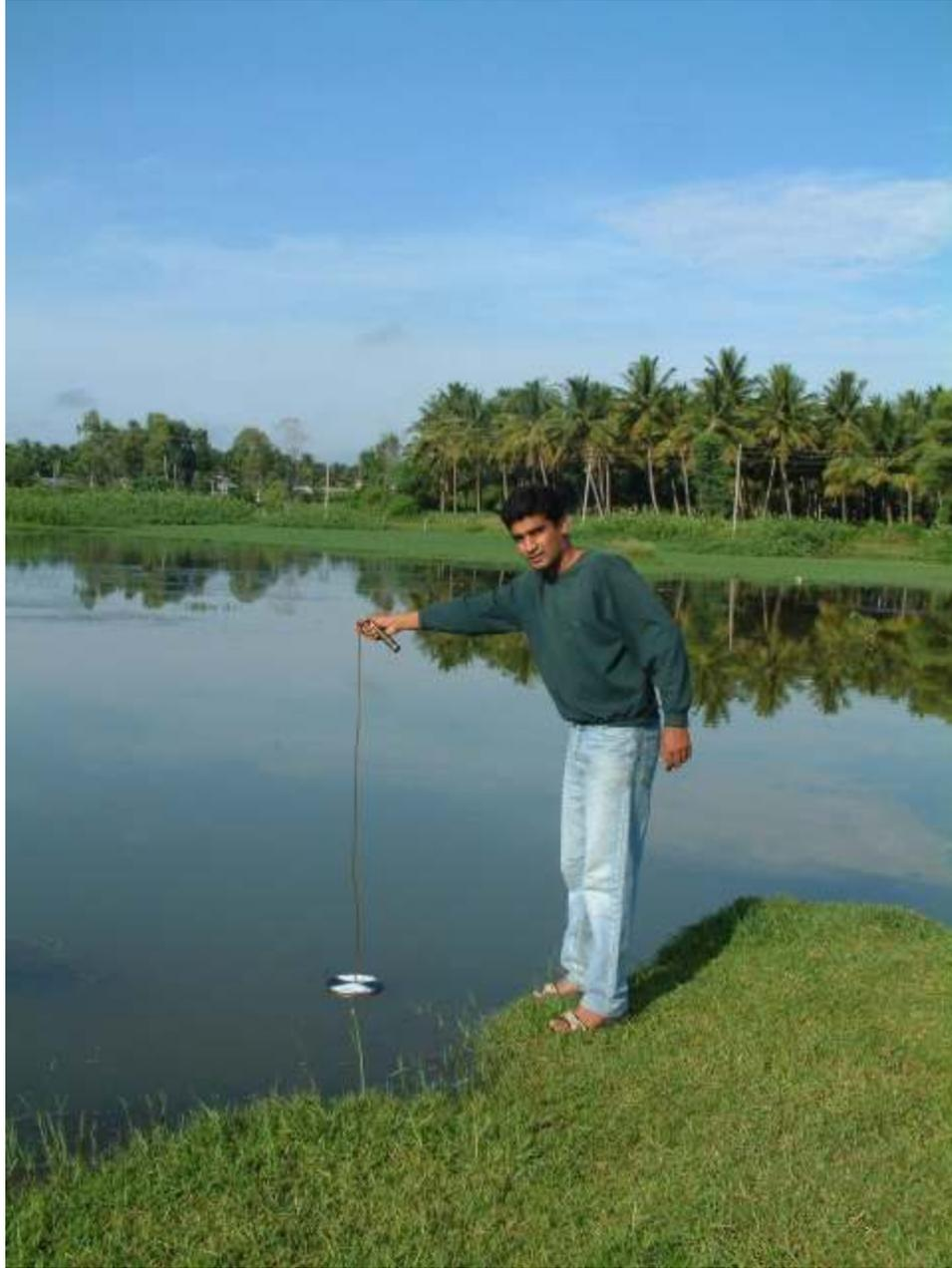
**Fig 2:** Measurement of Secchi Depth
