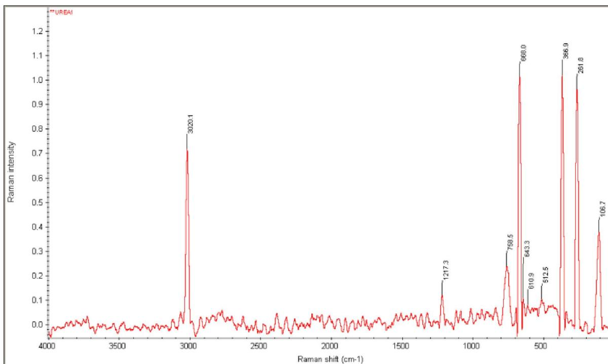
**Figure 04: Raman spectral acquisition of lipid sample**
