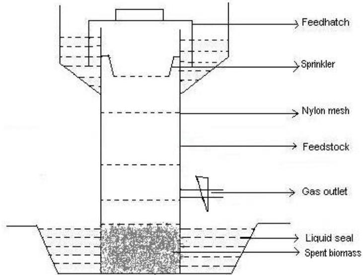
Fig 3.1. Sketch of SSB reactor.
