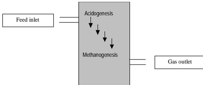
VFA's, inturn acted upon by the methanogens, results in the production of biogas. Acidogens present at the top portion of biomass bed, rapidly hydrolysing the polymeric substances results in the production of VFA, this inturn get in to contact with those methanogens at the bottom, is possible through leachate recycling process.
