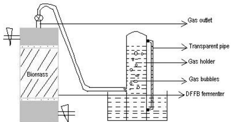
Fig 3.7. Sketch of DFFBR showing gas measured by downward displacement of water.
