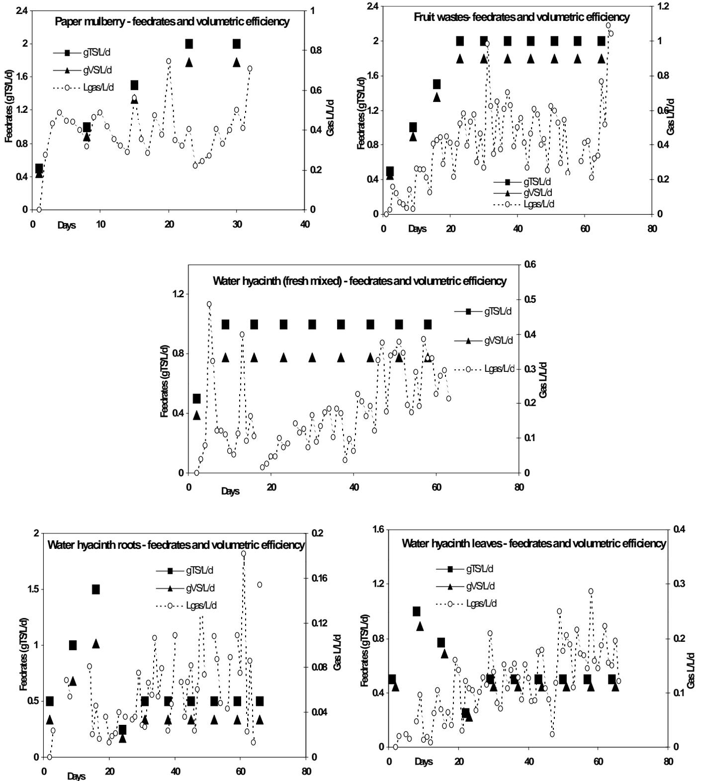
Fig 4.6. Feed rate Vs volumetric efficiency in fresh feedstock
