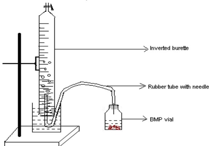
Fig 3.5. Sketch showing the set-up used for measurement of gas production from BMP vials
