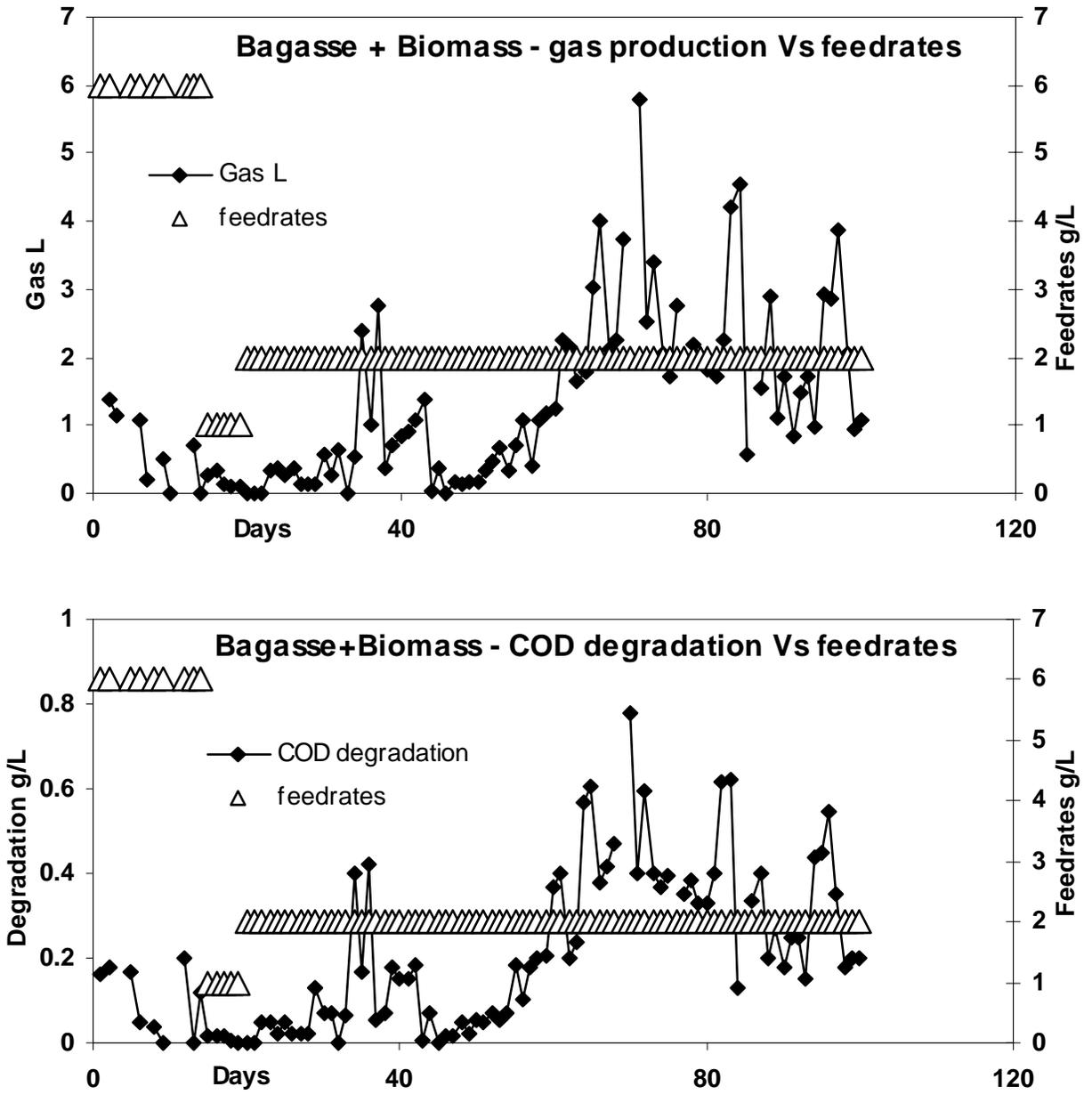
Fig 4.33. Feed rates Vs Gas production and COD degradation for bagasse + biomass
