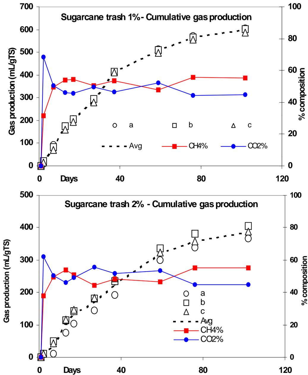
Fig 4.16. Cumulative gas production pattern of sugarcane trash.
