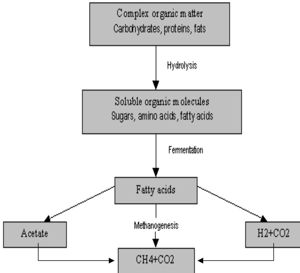
Fig 2.4. Overall scheme of anaerobic digestion process.
