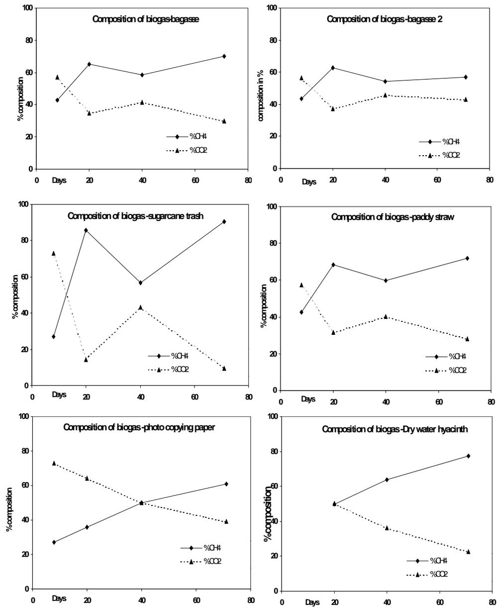
Fig 4.7. Composition of biogas in dry feedstock.
