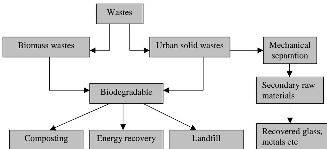
Fig 2.2. Pathways for solid waste treatment for recovery and recycling process.
