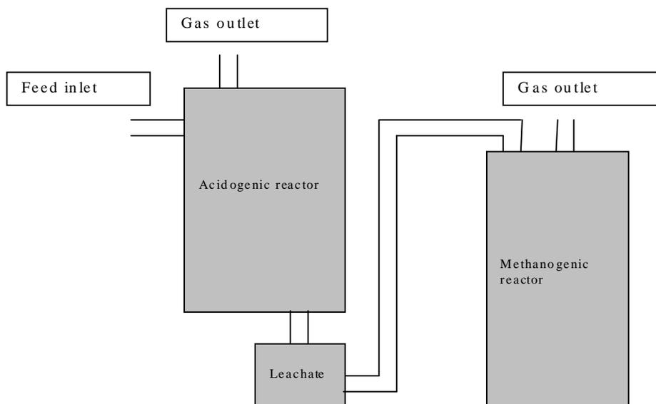
Fig 2.7. Two-step digestion
