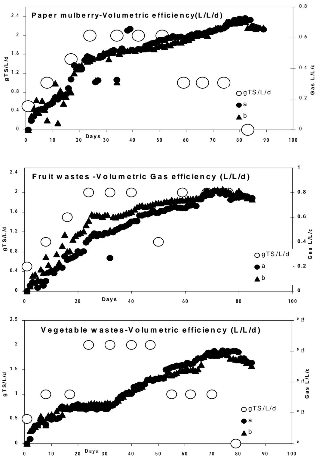
Fig 4.13. Volumetric efficiencies and gas production pattern of feedstocks in run 2 experiment
