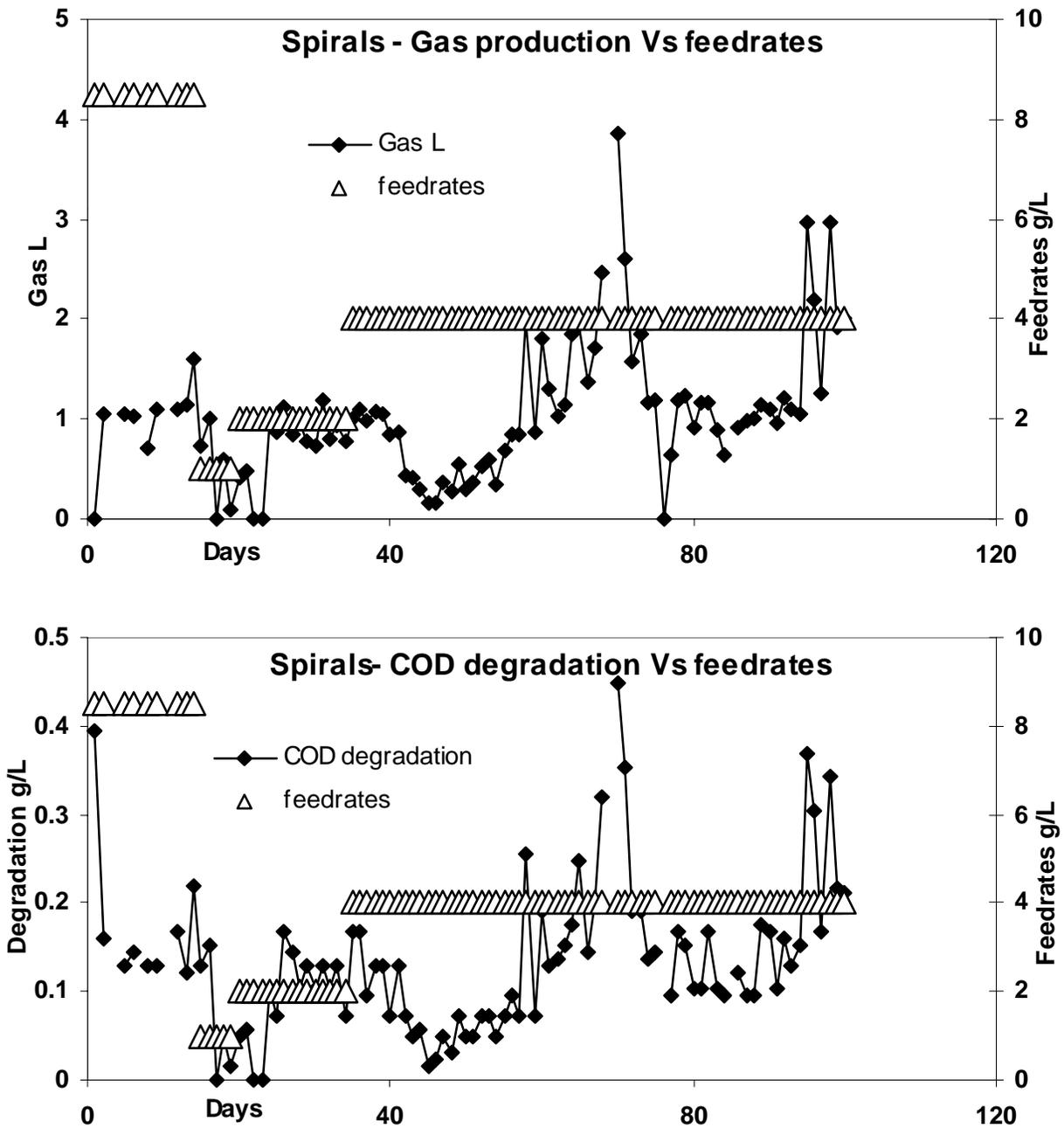
Fig 4.32. Feed rates Vs Gas production and COD degradation for spirals
