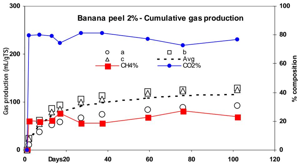
Fig 4.21. Cumulative gas production pattern of banana peel.
