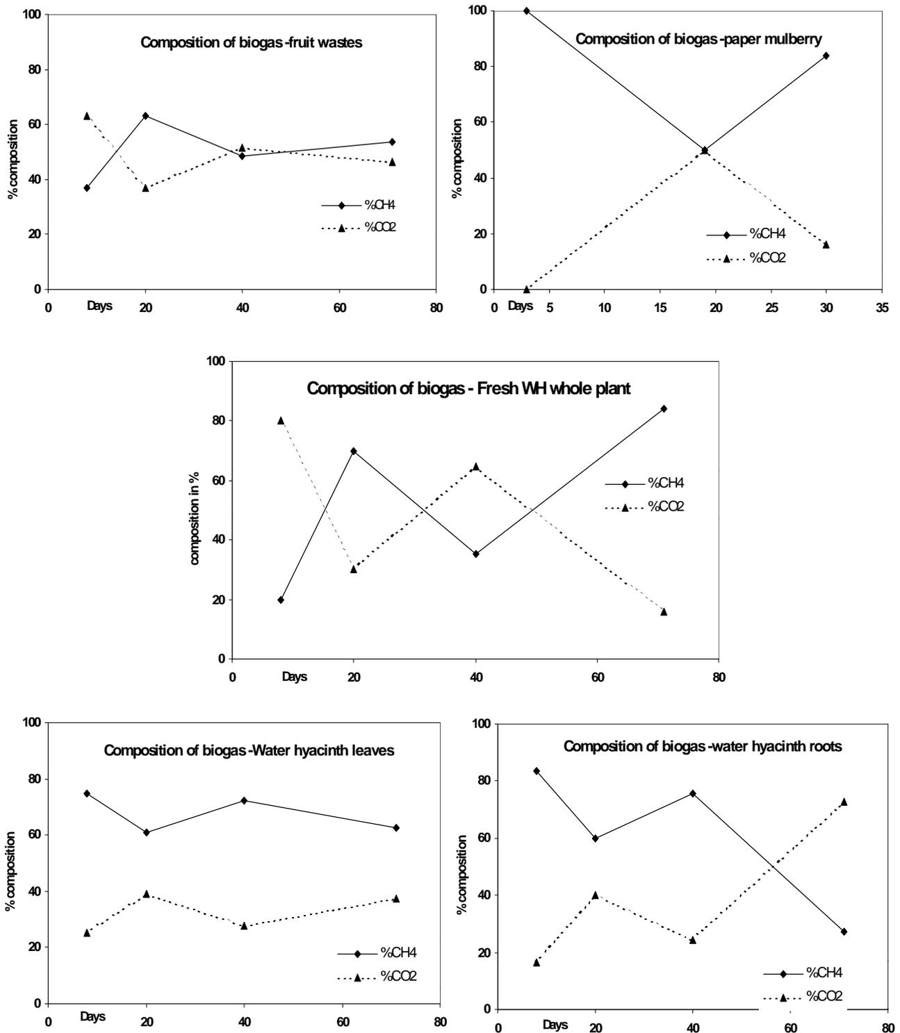
Fig 4.8. Composition of biogas in fresh feedstock.
