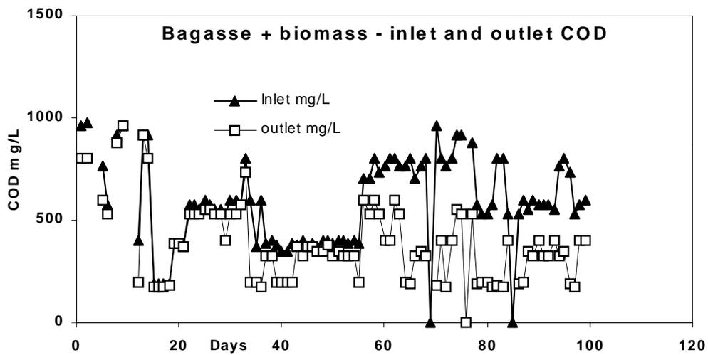
Fig 4.34. COD reduction in DFFBR reactor.
