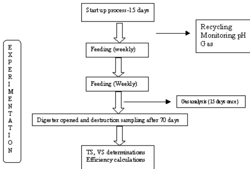
Fig 3.3. Overall experimental protocol
