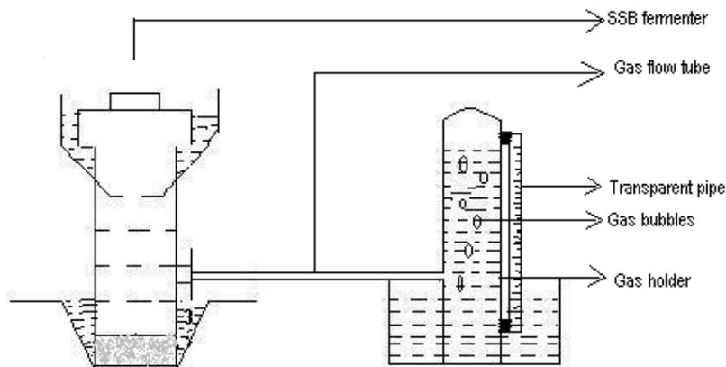
Fig 3.2. Sketch showing gas measurement by downward displacement of water.
