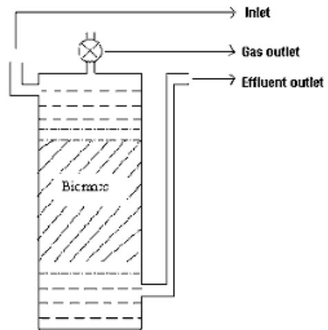
Fig 3.6. Sketch of laboratory scale DFFBR
