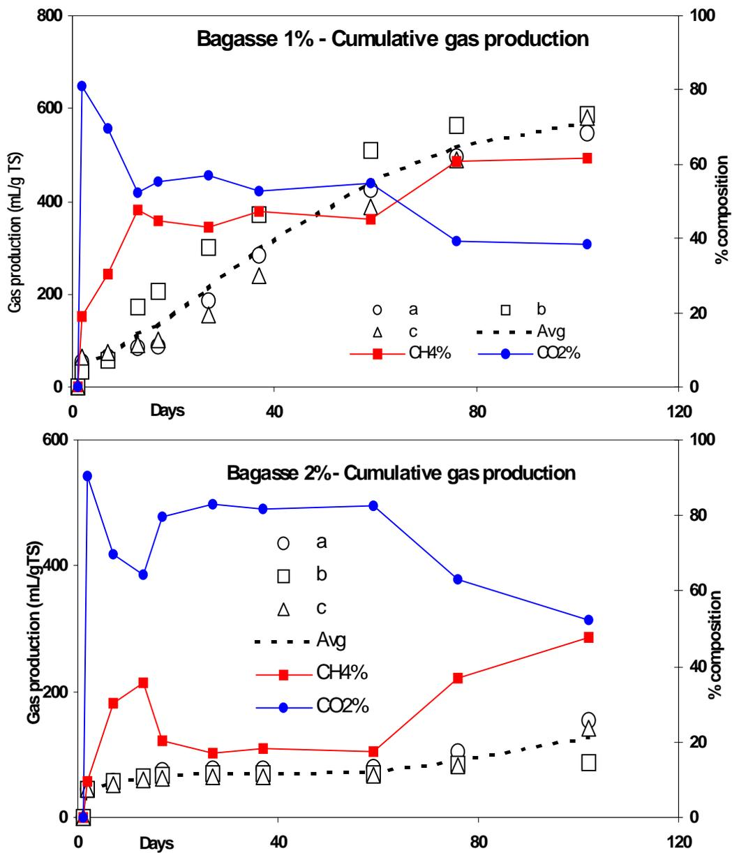
Fig 4.14. Cumulative gas production pattern of bagasse.
