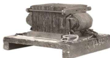
*A first prototype transformer built by Stanley in 1885*
