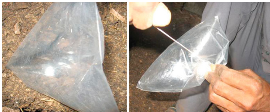
Fig. 6 Gas collection from compost plant
