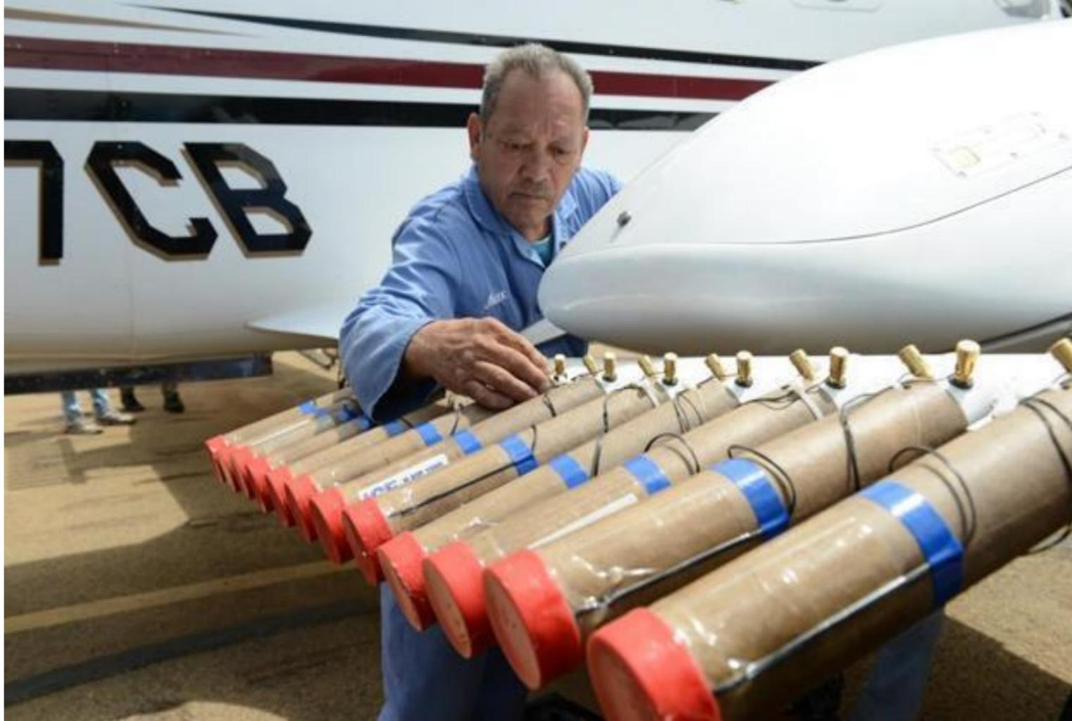
The Beechcraft King aircraft uses silver iodide, potassium chloride and sodium chloride—chemicals that can aid precipitation when seeded into rain-bearing clouds. Photo: Hemant Mishra/mint
